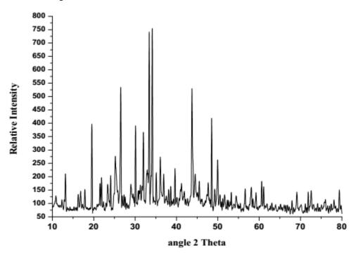
Fig 1: XRD structure of MgCuAl<sub>10</sub>O<sub>17</sub> Phosphor
